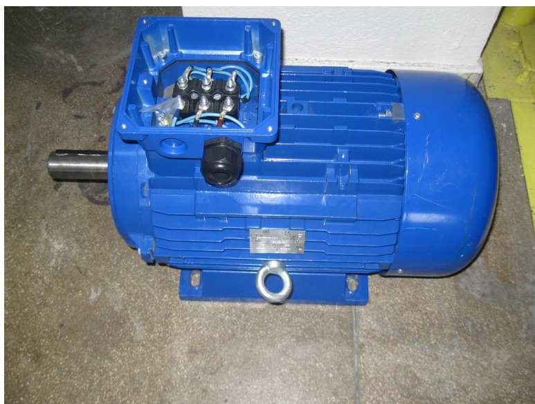
Motorul MAL160M-IE3-42-6A (7.5 kW – 1000 rot/min)
