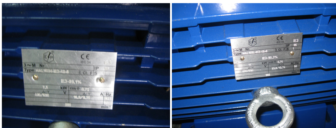
Fig.11. Motorul MAL160L-IE3-42-6B (11 kW – 1000 rot/min)
