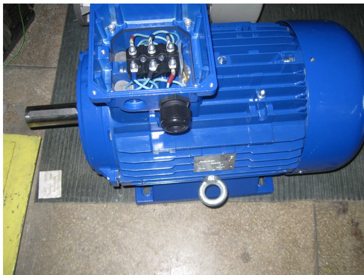
Fig.11. Motorul MAL160L-IE3-42-6B (11 kW – 1000 rot/min)
