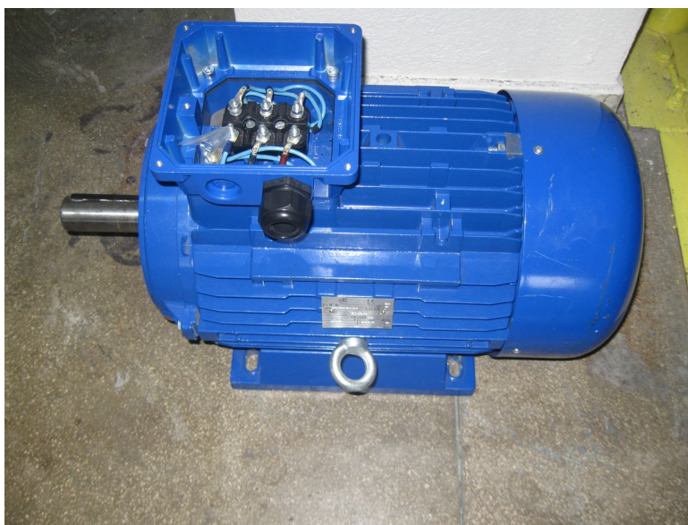
Fig.10. Motorul MAL160M-IE3-42-6A (7.5 kW – 1000 rot/min)
